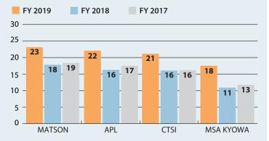
The container vessel net moves per hour (NMPH) shows the average total container movement divided by the operation hours. PAG's goal is to increase the number of containers in NMPH per year. In FY 2019, all vessels showed improvement by an average of six NMPH.
